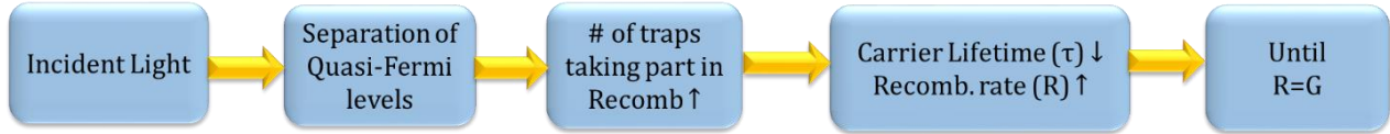
Fig. 4.12. Shining light on the cell will cause a photo-voltage to develop across the sample.
